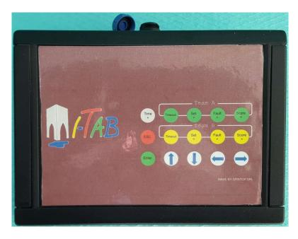
The console is able to remote control the scoreboard in a very efficient way because it has up to 15 dedicated buttons. Using wire connection, it can be placed up to 200m from the display, alternatively there is a RF version that do not need a cable and that can be placed up to 100m from display.
