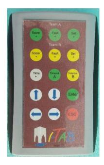
The remote control allows the referee or who for him to control the scoreboard by remote via radio. This device, as the console, comes with 15 keys that let you perform operations with greater efficiency.
